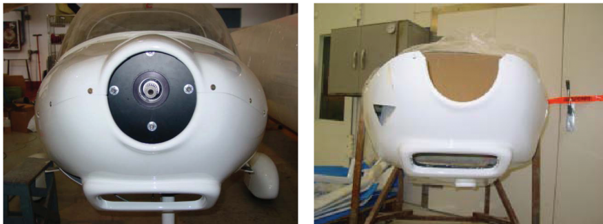
Fig. 8 Lower cowling modification.
