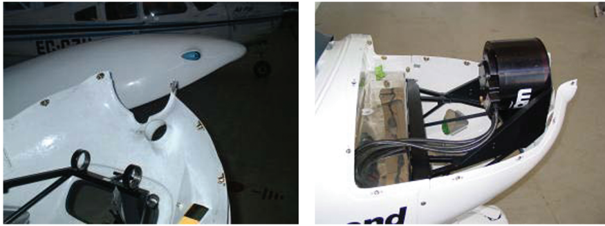
Fig. 6 Engine tray modification.
